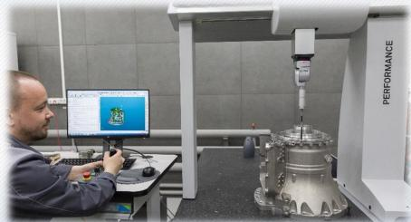
**PC-DMIS** software allows to evaluate geometry of parts and generate a detailed inspection report with various visualization possibilities. **Quindos GEAR** is used to control geometry of involute splines and gears manufactured according to **GOST, ISO, DIN** standards. Inspection can be made for spur and helix gears, outer and inner toothing.
